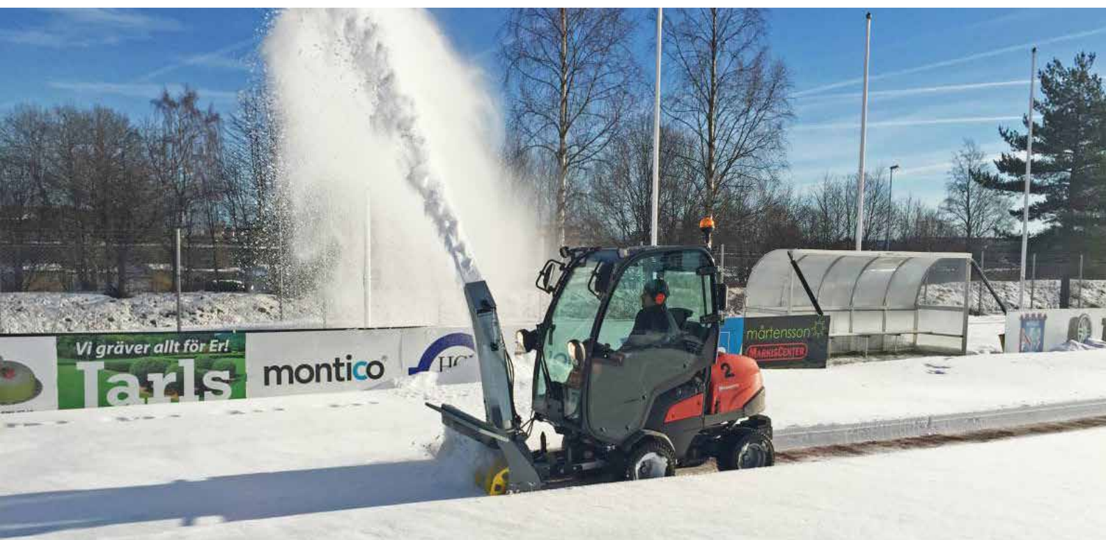
SNOW BLOWER ON A HUSQVARNER OUT FRONT MOWER
